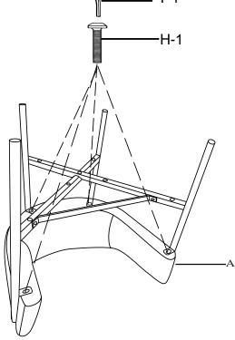
Put Back Cushion(A) upside down onto a padded, non-marring surface. Position the assembled frame on the Back Cushion(A) and loosely secure with Medium Bolts(H-1) using provided Allen Wrench (T-1). Do not yet fully tighten bolts.
