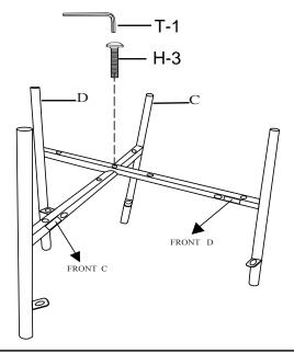
Cross the Upper Frame(C) and Bottom Frame(D) as shown. Loosely secure with Long Bolt(H-3) using provided Allen Wrench(T-1). Do not yet fully tighten bolt.
