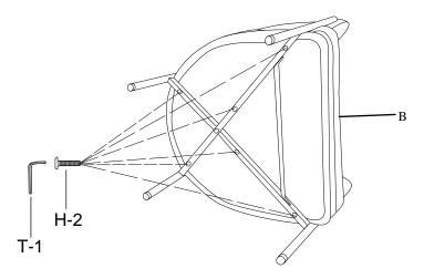
Lay assembly on its side onto a padded, non-marring surface. Position Seat Cushion (B) onto assembly as shown and loosely secure with Extra Long Bolts (H-2). Do not yet fully tighten.
