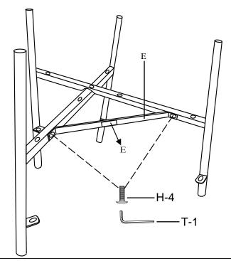
Position Stretcher Rod(E) on the front of the assembled frame as shown. Loosely secure with Small Bolt (H-4) using provided Allen Wrench(T-1). Do not yet fully tighten bolts.
