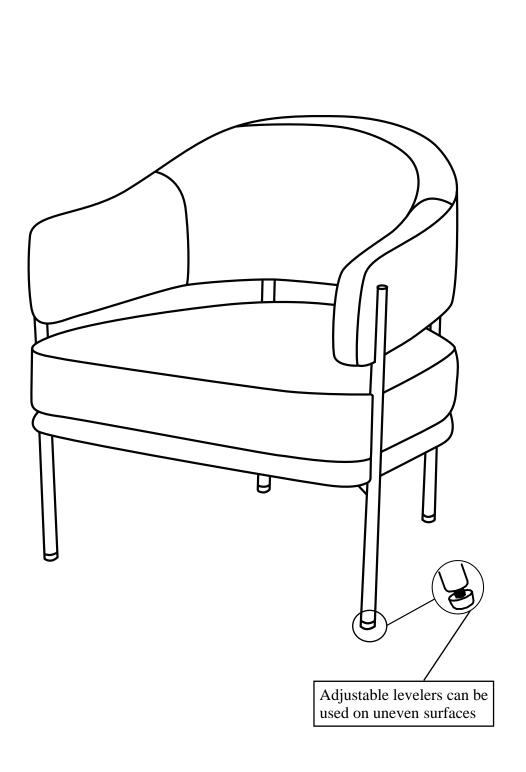
Carefully turn assembly upright, ensuring it rests evenly and level on all 4 legs. Fully tighten all bolts from Steps 1-4 at this time using provided Allen Wrench (T-1). Assembly is now complete and products ready for use.
